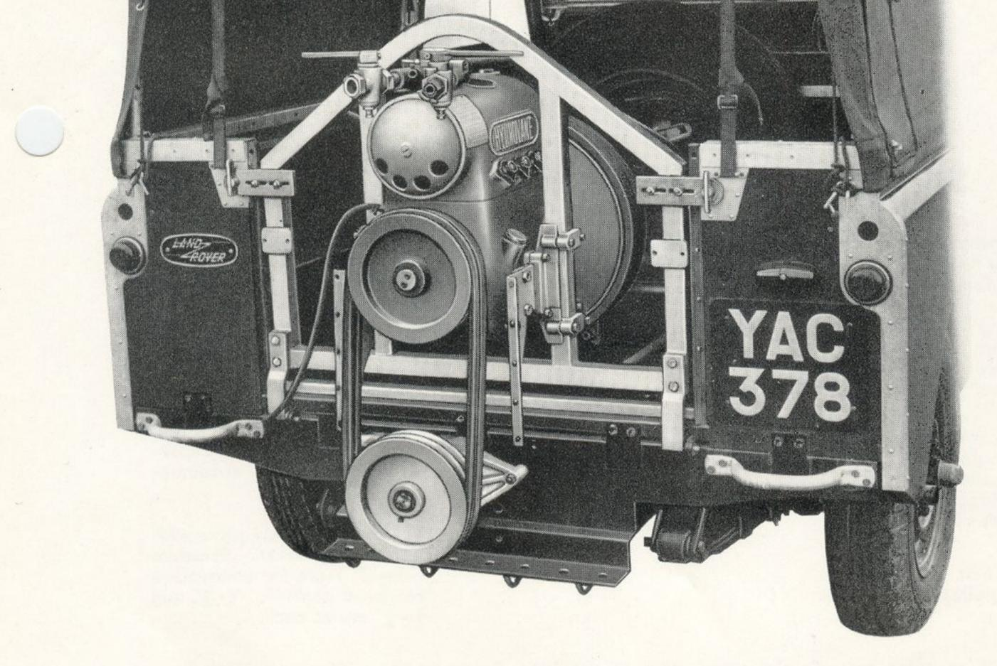
and valves and has no external pipework other than from the compressor to the speed control at the engine end. Incorporated in the compressor is a servo valve mechanism which gives a pressure drop of 2-3 p.s.i. only between no flow and full flow conditions.
