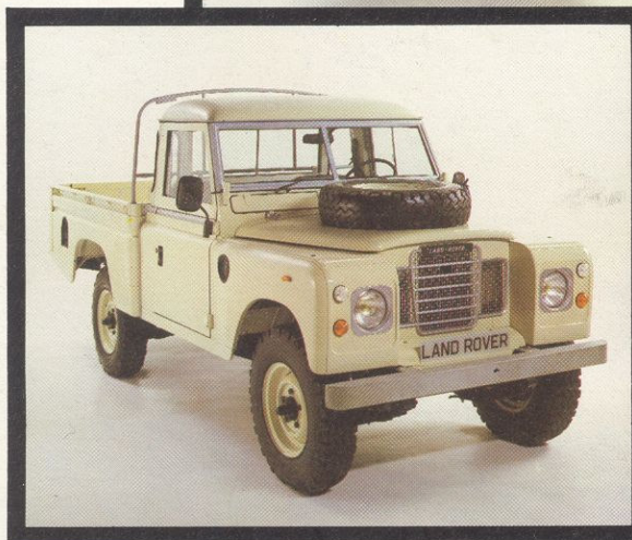
Bed length A = 2.01m (79") Bed width B = 1.63m (64") Bed width C = 0.92m (36")
