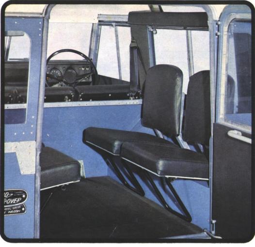
Three front seats are also provided in the the vehicle. A folding mounting step is 7-seat Station Wagon. Trimmed and pad-provided to assist entry.
