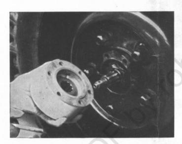
6. Fix the new paper gasket to the flanged face of the free-wheeling hub main unit with jointing compound or grease. Check that the pawls are fully engaged. Locate the centre gear of the main unit on to the splined stub axle, push home and loosely screw in one bolt to hold it in position.
