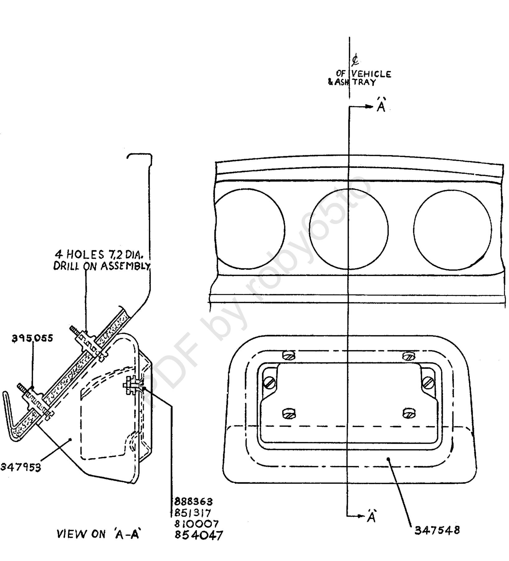
Fig. 1. Ashtray fitted to the sloping front face of the parcel tray
