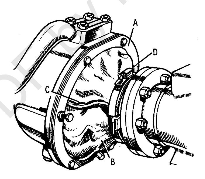
Fig. 1. Gaiter fitted to swivel housing.
