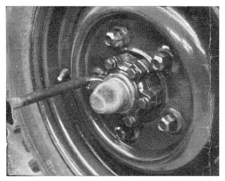
1. Remove the oil cap covering the extension of the front stub axle.
