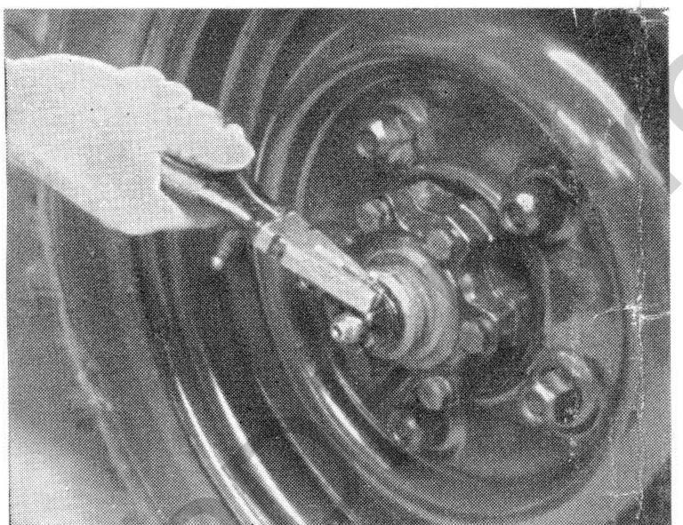
2. Remove the cotter pin securing the castellated nut on the extension of the stub axle.
