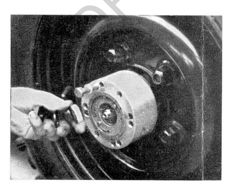
7. Fit the new rubber and felt oil seal with washer on the splined stub axle and screw on the original castellated nut. DO NOT OVERTIGHTEN, i.e., first tighten the nut and turn back to the nearest position for the cotter pin to be inserted and spread.
