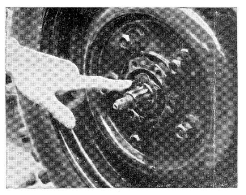
5. Jack up the vehicle at the front and check whether there is any end float on the wheel bearings. If so, correct before proceeding any further. (The Land Rover Manual should be referred to — operation F16 in the Series 2 manual.) The end float is removed with inner hub nut and lock-nut. As a safeguard this should be checked again after locking the lock-nut in position.
