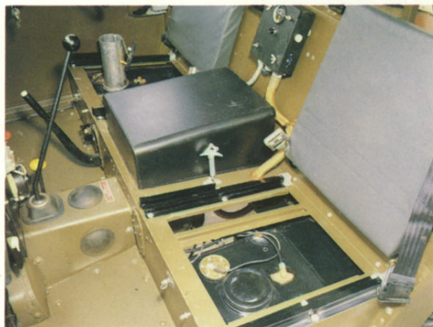
Twin underseat fuel tanks.
