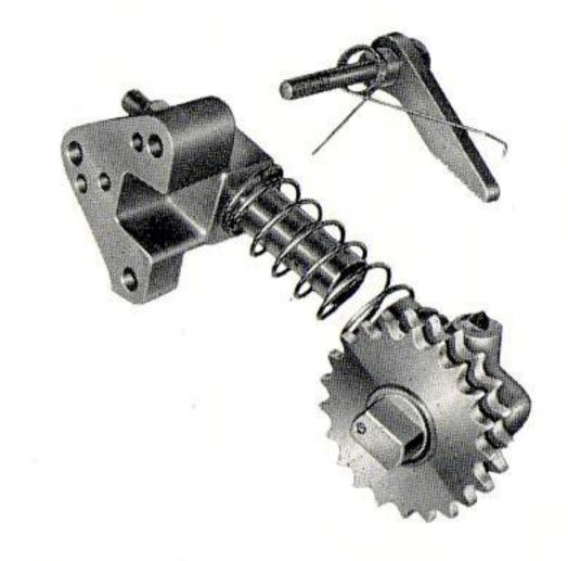
prevents the chain from slackening. A rubber damper pad is also fitted on the taut side of the chain to prevent whip.
