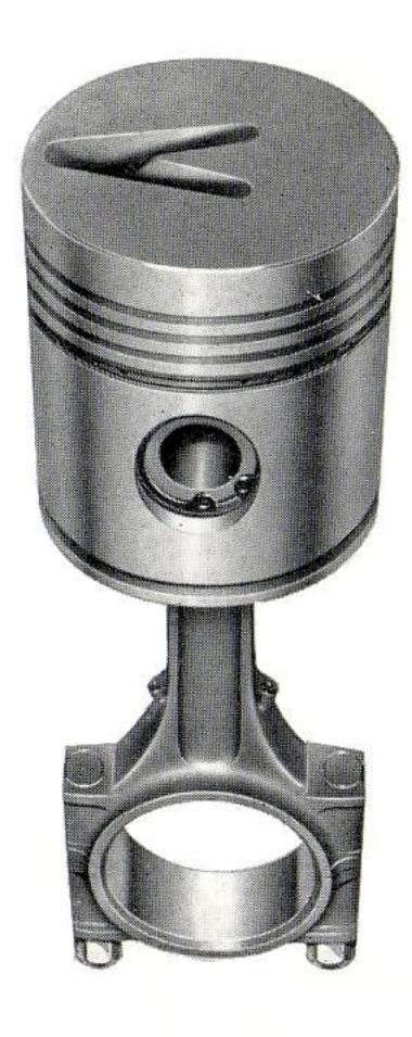
Connecting rods are of forged steel and incorporate a jet hole through which oil from the big-end bearings is squirted on to the thrust side of the cylinder walls. The upper part of the big-end is so made that piston and connecting rod may be withdrawn upward through the cylinder bores to facilitate servicing.
