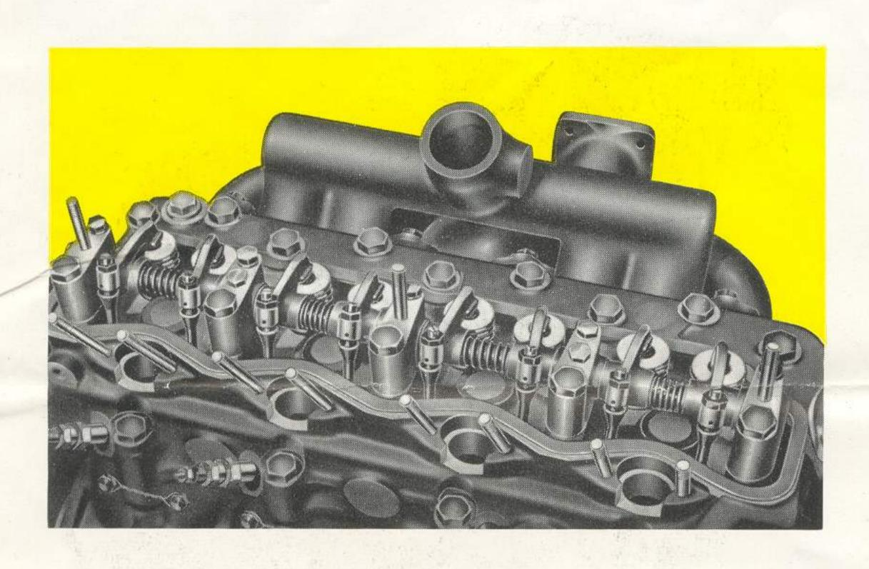
The overhead valves are operated by push rods and rockers from a chain-driven camshaft. Valve heads are of large diameter to give the most efficient breathing and they are cooled by ample water passages between the ports.
