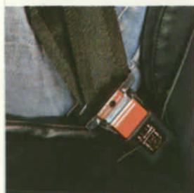
Above. The front seat belts are of the static, single-handed type.
