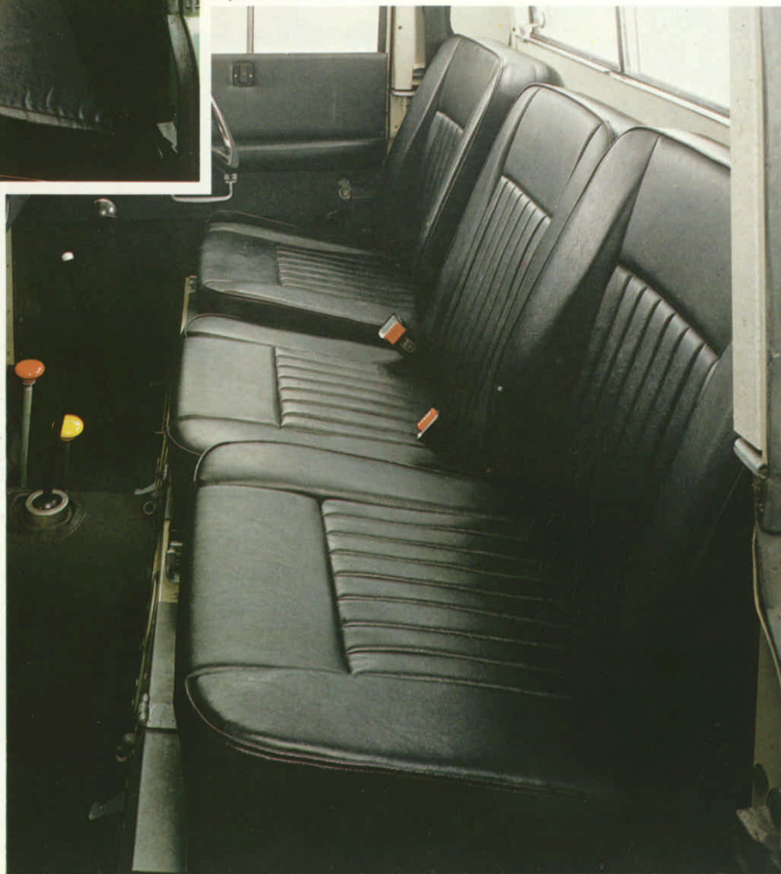
Above. The front seat belts are of the static, single-handed type.
