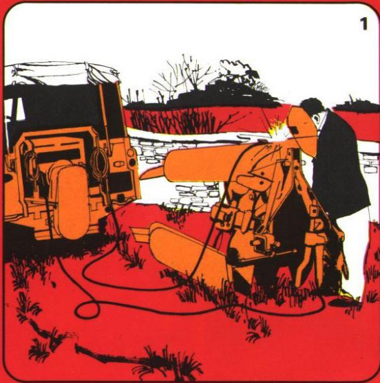
1. The Land-Rover makes an excellent basis for portable welding sets, and several types are available, making it virtually unbeatable for fast on-site welding.
