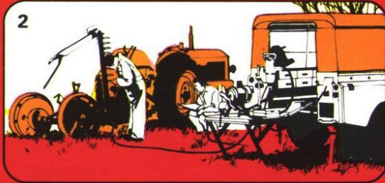
1. The Land-Rover makes an excellent basis for portable welding sets, and several types are available, making it virtually unbeatable for fast on-site welding.
