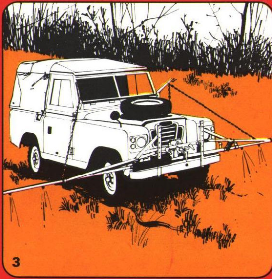
3. For roadside verges, parks, golf courses and other grassed areas, a Land-Rover spraying unit covers the ground quickly and economically.
